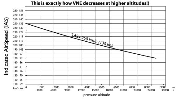
**WARNING!** Above pressure altitude of 4000 meters (13100 ft) VNE (see previous page) MUST be treated as True AirSpeed (TAS). Indicated AirSpeed (IAS) MUST be reduced accordingly! Table with IAS, TAS relation for 302 km/h (163 kts) is below:
