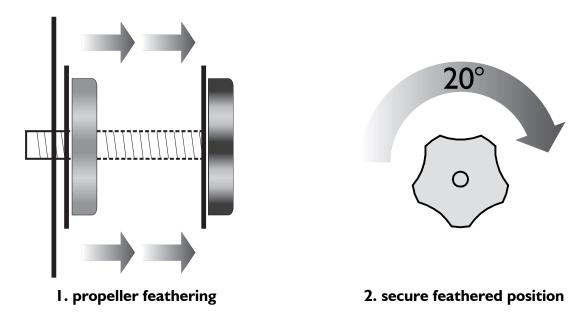
**WARNING!** Feather propeller only after the engine has stopped and at minimum pitch.
