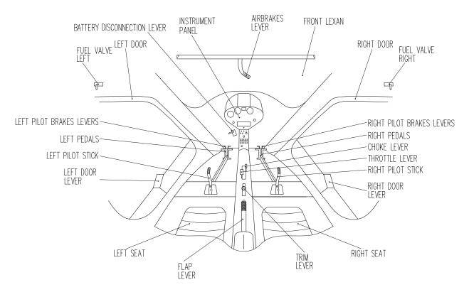
Individual control levers: pilot stick and rudder with belonging brake levers
